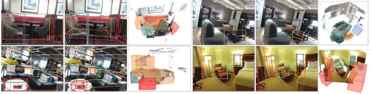
Figure 2.21: Some failure cases. The perspective point estimation and the 3D box estimation fail at the same time.
