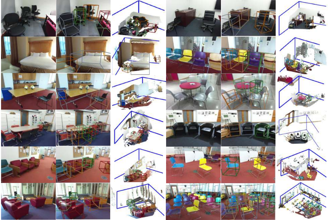
Figure 2.13: Qualitative results (top 50%). (Left) Original RGB images. (Middle) Results projected in 2D. (Right) Results in 3D. Note that the depth input is only used to visualize the 3D results.
