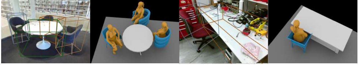
Figure 1.2: Human-centric 3D scene parsing and reconstruction. By incorporating imagined humans into the task-oriented computational framework, the perception system can generate interacting humans and infer the affordance of the reconstructed 3D scenes. (from [HQZ18])
