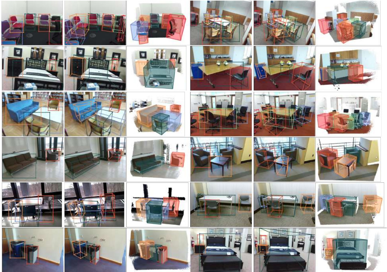
Figure 2.18: Qualitative results (top 50%). For every three columns as a group: (Left) The RGB image with 2D detection results. (Middle) The RGB image with estimated perspective points. (Right) The results in 3D point cloud; point cloud is used for visualization only.
