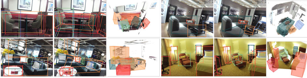
Figure 7: Some failure cases. The perspective point estimation and the 3D box estimation fail at the same time.
